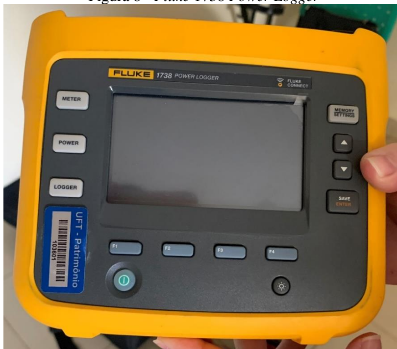
Figura 8 - Fluke 1738 Power Logger
